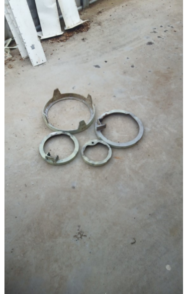
Right: The boom bulkheads removed, cleaned and ready to be sent of for assessment in Brisbane
