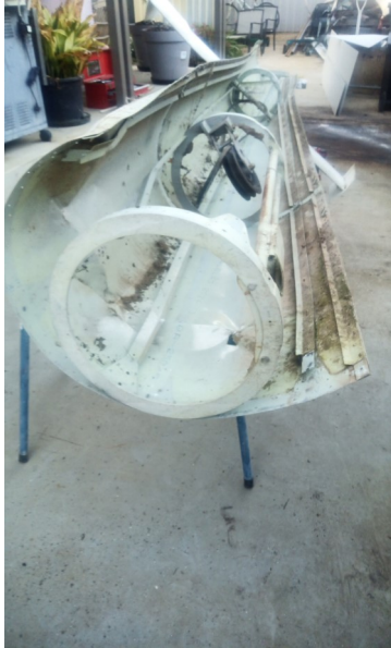
Left & Right are pictures of the partly dismantled tail boom, bulkheads visible after removal of about 200 "Cherry" rivets.
