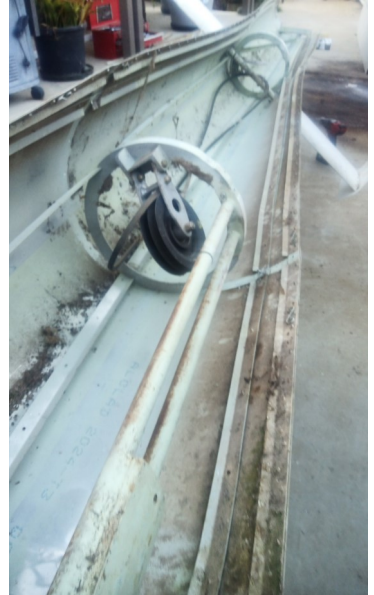
Left & Right are pictures of the partly dismantled tail boom, bulkheads visible after removal of about 200 "Cherry" rivets.
