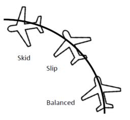
Let's go back to the second diagram. Right bank, enough left rudder to stay straight. What are the instruments telling you?
