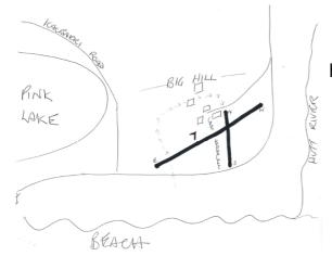
NOTE: If using North/ South strip a tight right hand circuit below hilltop and between houses is required.
