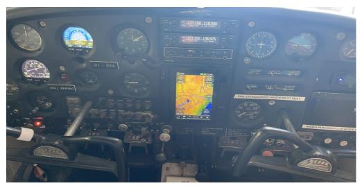
Just to recap, I have fitted a new Attitude indicator (AH), Directional Gyro, both of which are Uavionix AV-30s, I have moved the old "steam engine" gyros across to the co-pilot side.
